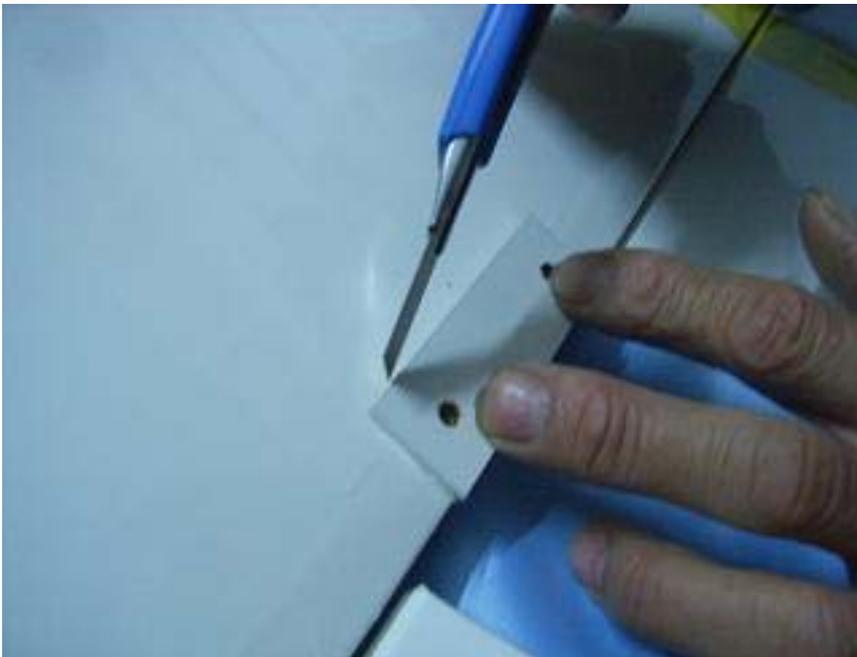
Find out the holes for the screw and remove the covering, referring to the small plywood's shape.
