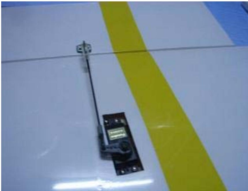
Fix the tri-horn at the right position, and connect it to the servo by pushrod.
