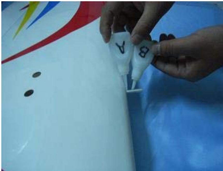
Use A.B. glue to the joiner and then insert it into the fuselage.
