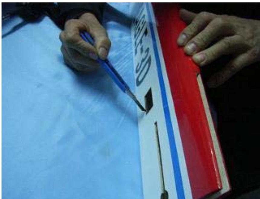
Find out and cut the hole for the elevator servo.
