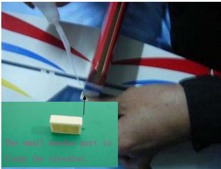
Insert the small wood part, and glue it to the fuselage to fixup the stabilizer.
