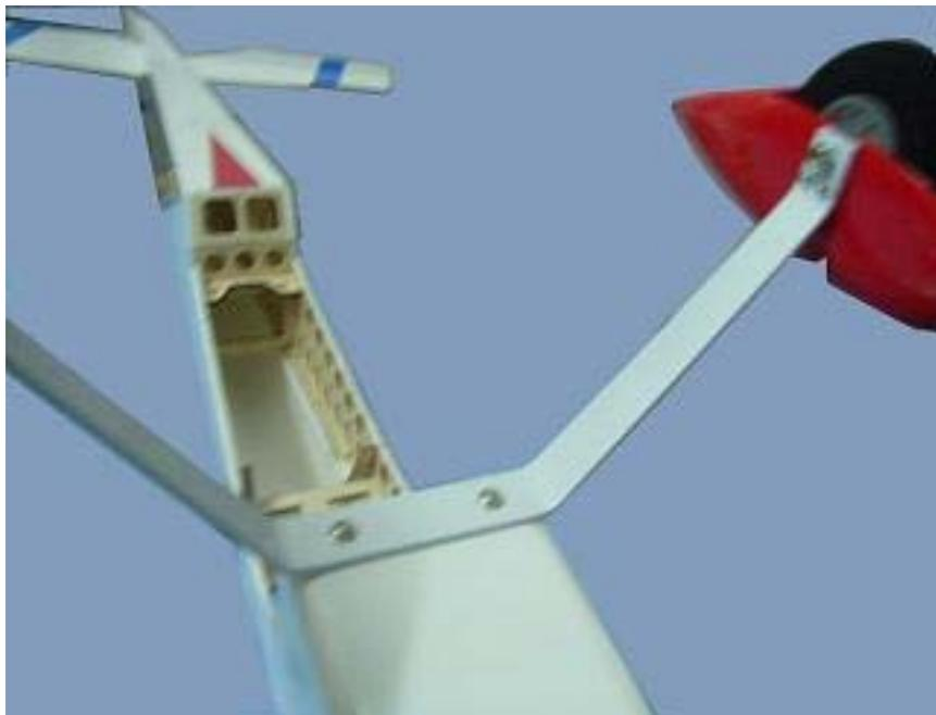
Screw the landing gear to the fuselage by two screws.
