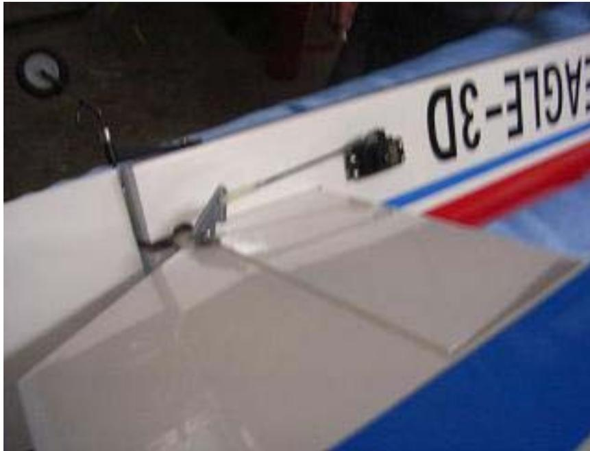
Install the elevator servo as shown.
