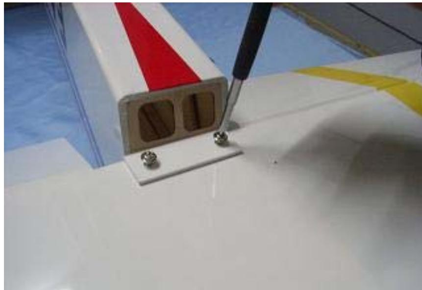
Fixup the wing to the fuselage by two screws.
