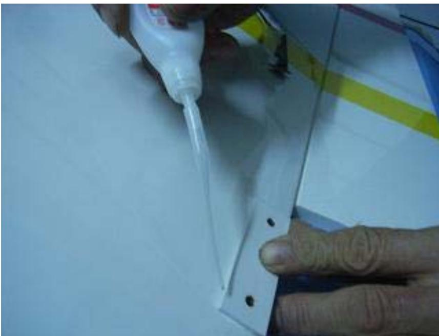
Glue the plywood to the main wing surely. Be sure the holes are in a line.
