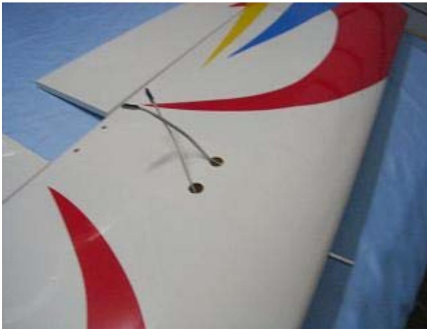
Pull the servo extension out from the holes in the main wing.
