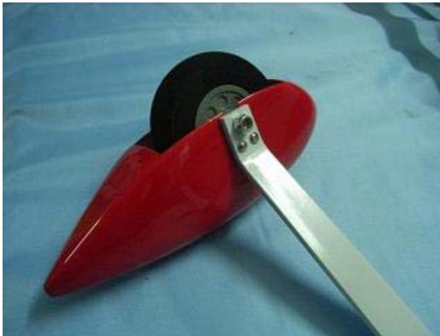
Fixup the wheel, wheel cover and the landing gear together.
