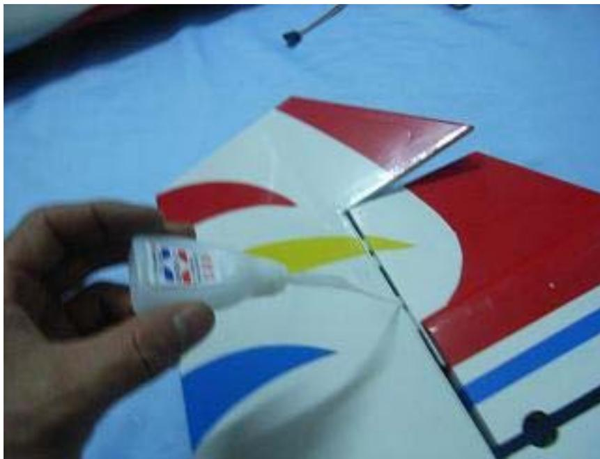
Connect the vertical fin and the rudder by hinges and glue them together.
