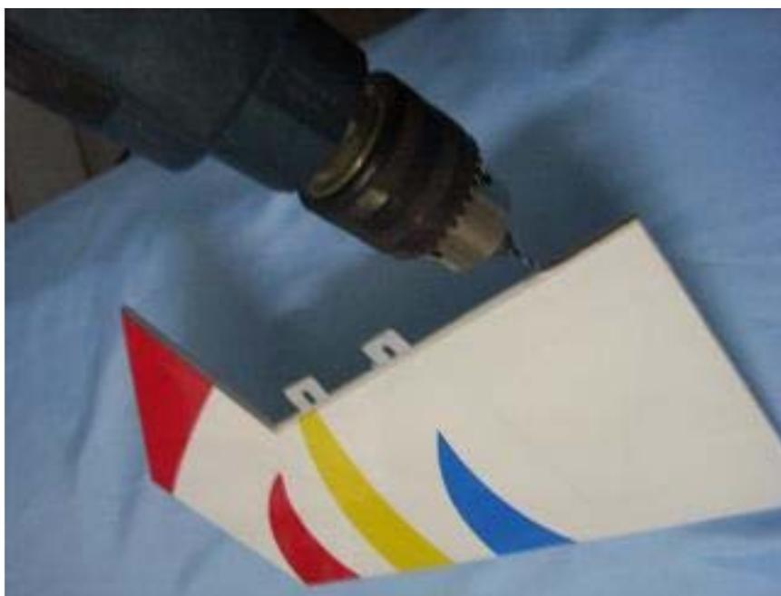
Drill hole for the tail wheel landing gear to insert into the rudder.
