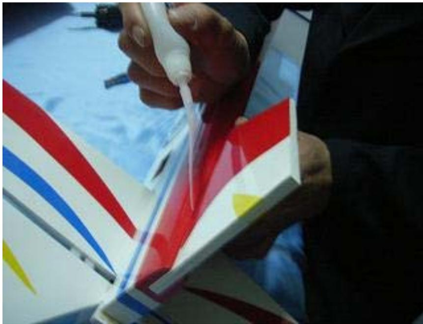
Glue the vertical fin to the fuselage.
