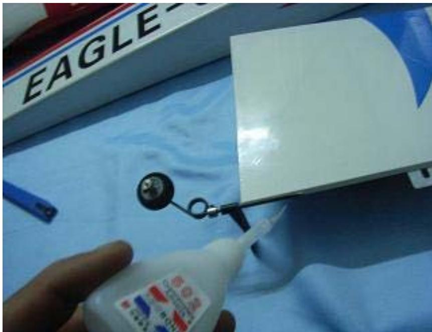
Insert the tail wheel landing gear into the rudder and glue it.
