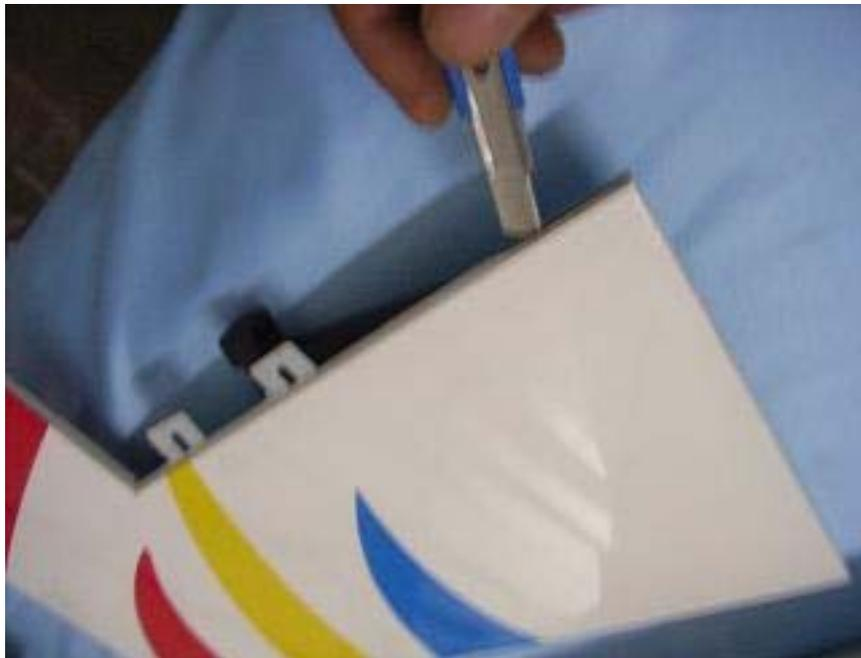
Remove the covering from the rudder for the tail wheel landing gear.
