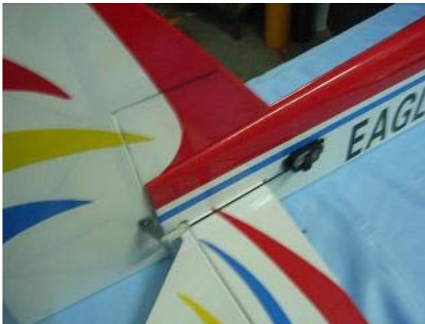
Install the rudder servo as shown.
