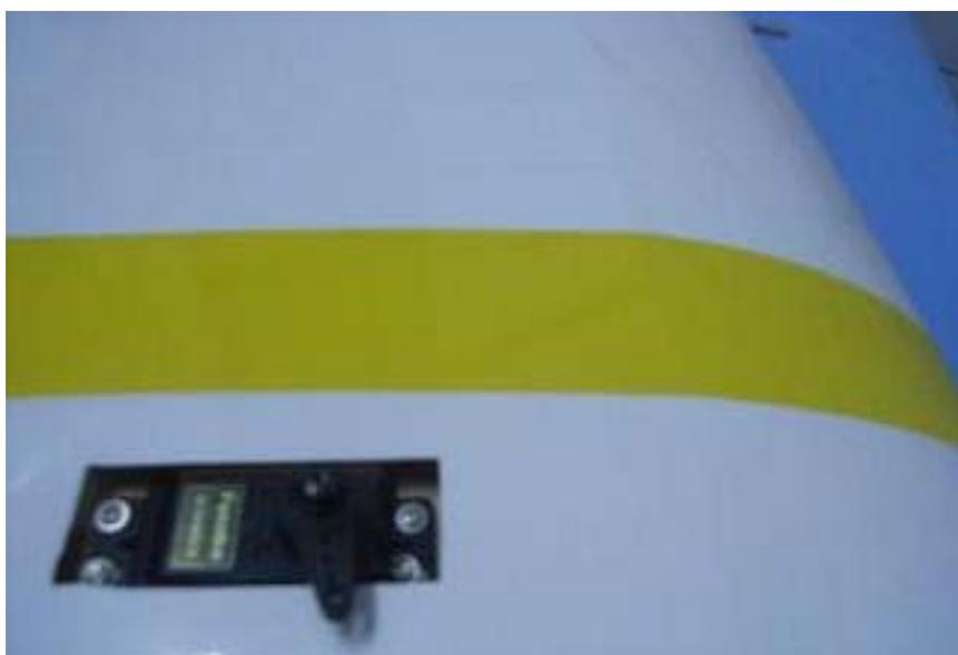
Fixup the servo by four TP screws.
