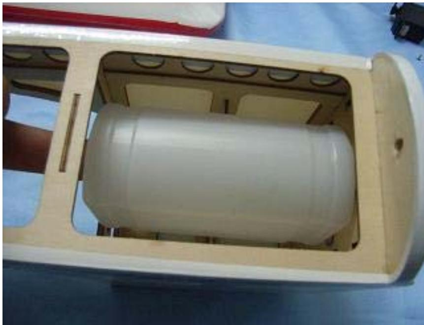
Put the fuel tank into the right position.
