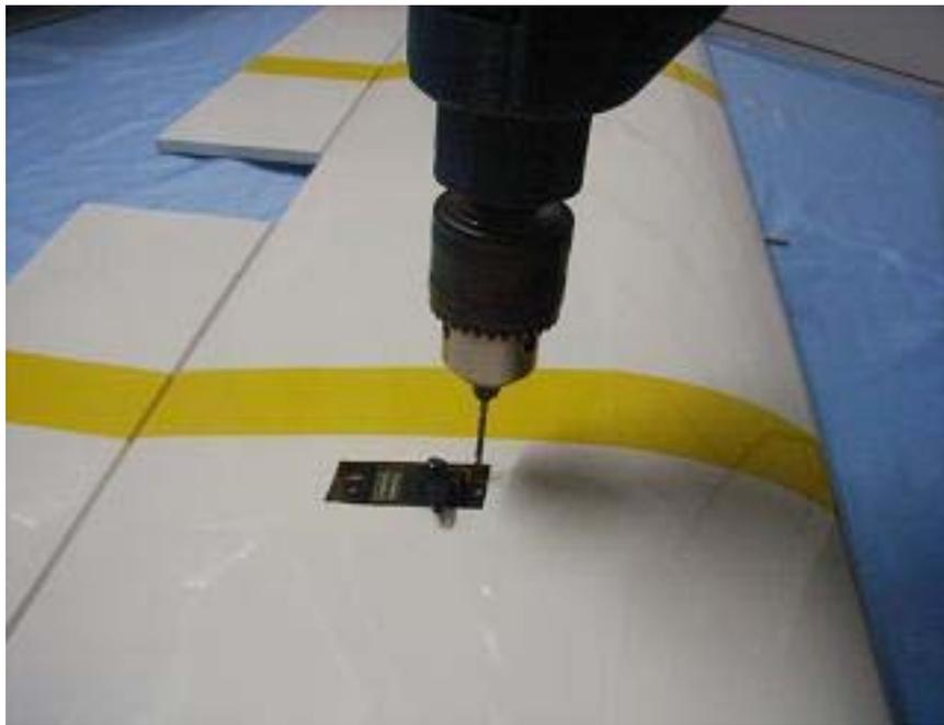
Put the servo into the hole, and drill holes for the servo screw.
