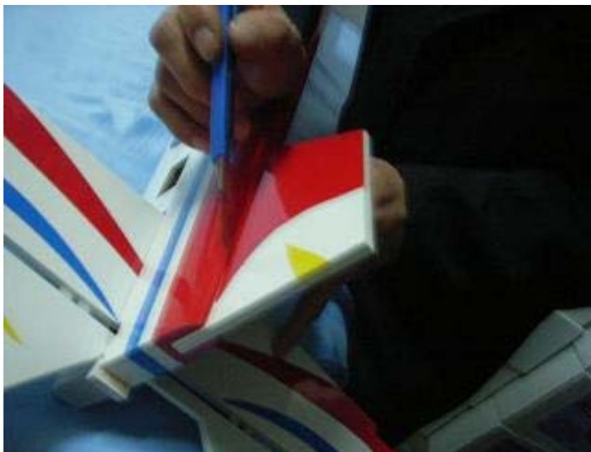
Measure and remove the covering from the vertical fin.
