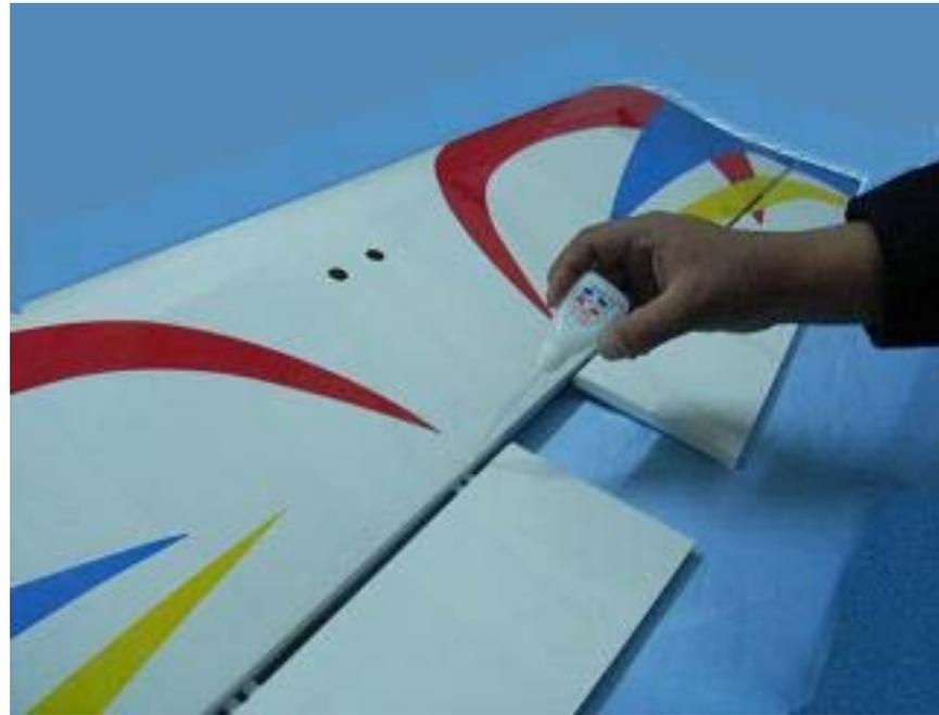
Connect the main wing and the aileron with hinges, and glue them to ensure its safty.
